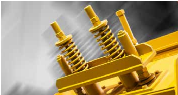
Manual crushing gap adjustment with spring system
