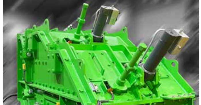
Full hydraulic gap adjustment
