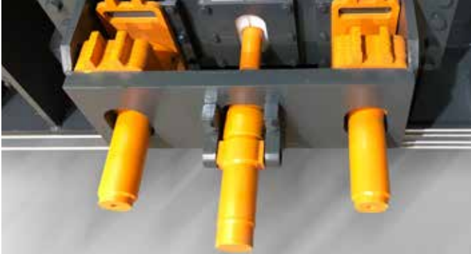
Grinding gap adjustment with spacer plates and hydraulic support
