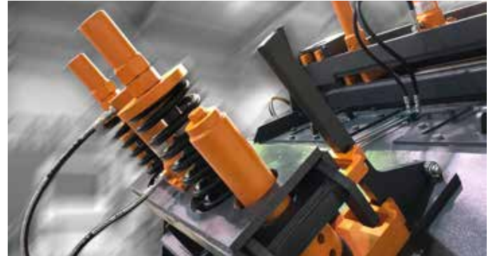
Crushing gap adjustment with spacer plates and hydraulic support
