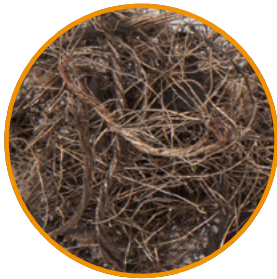
Tire wires after pre-shredder/granulator but with a large rubber content
