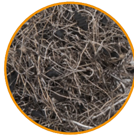
Tire wires after PTV - Delamination of wire and rubber in one pass around 99%
