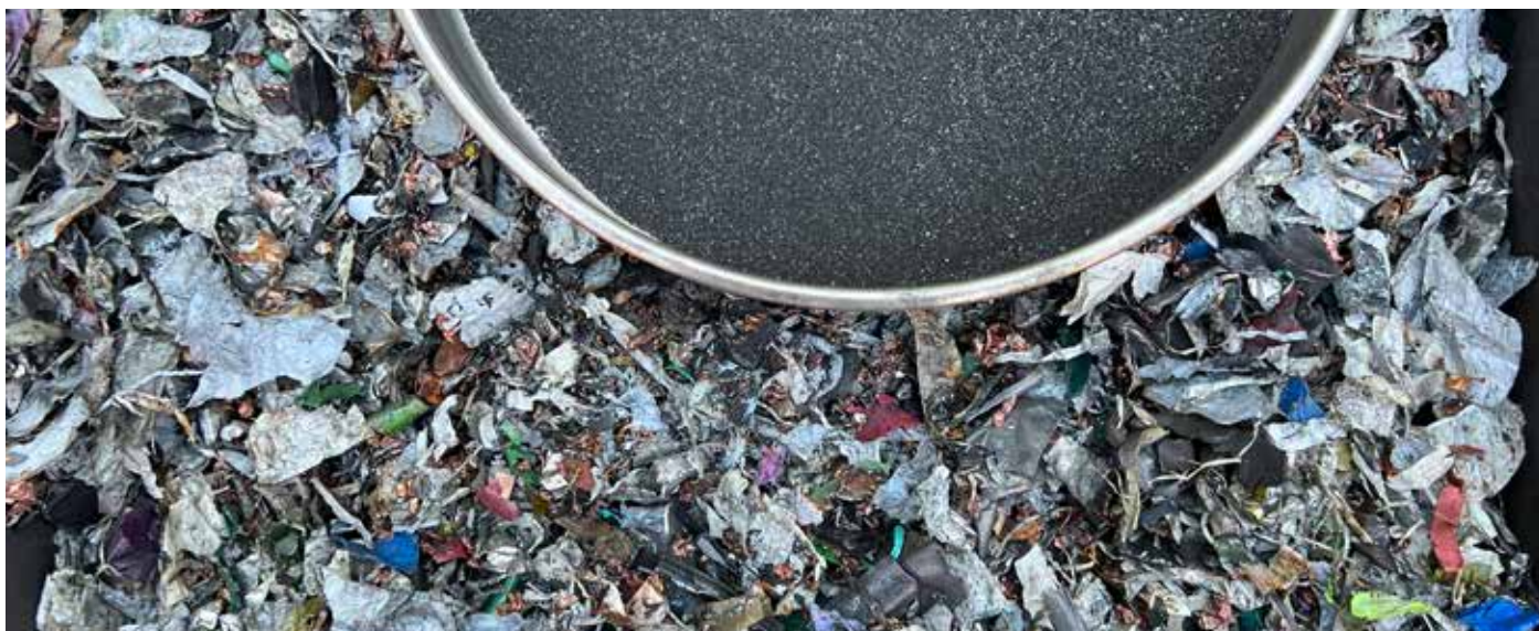
BATTERY BREAKDOWN & BLACK MASS LIBERATION
