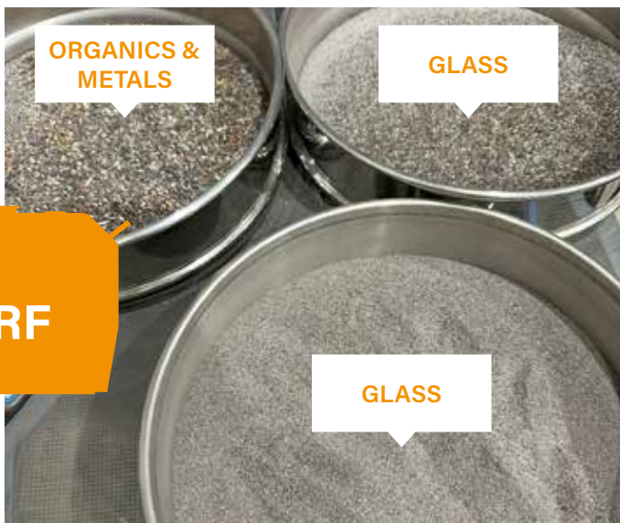
OUTPUT MATERIAL AFTER PTRF FINE GRINDING MILL & SIEVING
